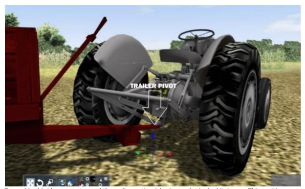
To enable this I have constructed the trailer so that it's pivot point is the hitch eye. This enables you to attach the trailer and then rotate it around the hitching point to enable it to go around corners or up and down slopes without trying to solve a complicated three dimensional headache. It also allows the trailer to be "parked" on its parking foot under the hitch.
