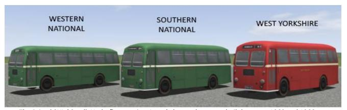
The Bristol SUL (Small, Underfloor engine, Long) shown above was built between 1960 and 1966. The bodies were again by ECW and this model is the B36F 36 seater. These buses were suited to rural areas being narrower and shorter than the MW models.
