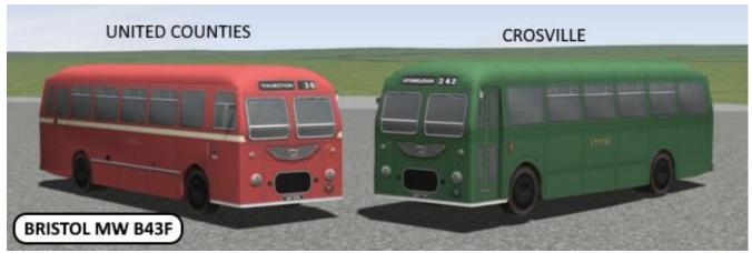
The MW B43F body was a 43 seater and is identifiable by the continuous roof profile at front and rear. This means the destination boards are smaller and set alongside each other. In every other external respect it is identical to the MW B45F model.
