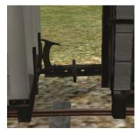
The Southwold Railway used a fairly simple chopper coupling. I have added a set of these to the wagons and they seem to work pretty well.
